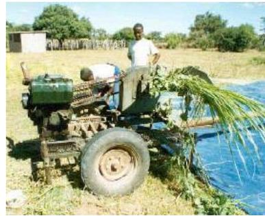
Figure 5. Diesel driven forage chopper
