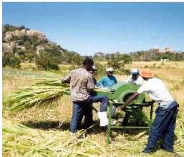
Figure 4. Feeding a hand driven chopper
